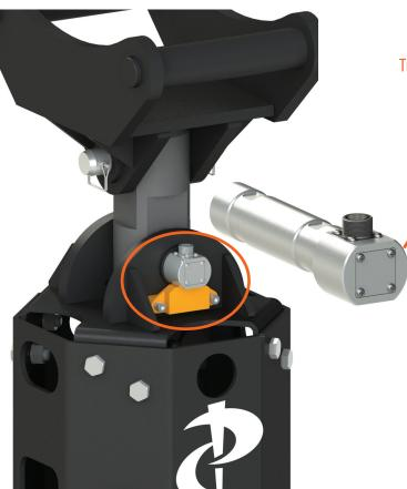
The TruLink™ Torque Monitor system offers true torque readings that deliver a high degree of accuracy (+/- 2%) while providing the operator with real time data. TruLink™ records actual torque being applied to the helical pile, the installation angle and the depth.
